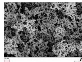
Multi layered **CVD3<sup>o</sup>Graphene™** covering the sintered Ni cellular material substrate made from Ni powder.
