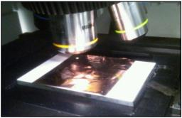
2"x2" Cu foil (Alfa Aesar, 99.8% purity), 25 µm thick
