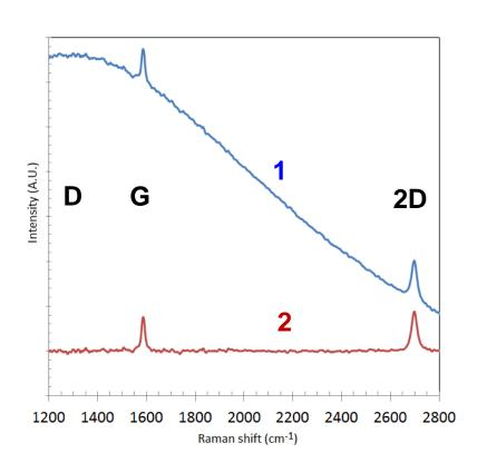
raw signal on as-grown CVD Graphene with important background owing to Cu fluorescence
