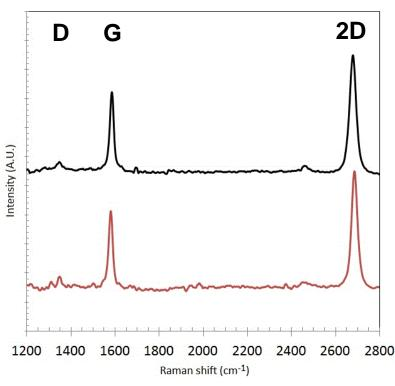
baseline corrected signal obtained for as-grown graphene on Cu foil
