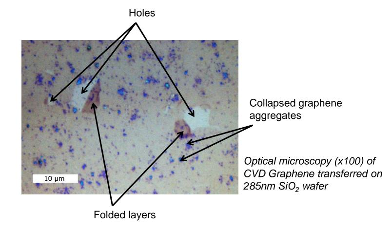
How to prevent any *misinterpretation* on the quality of graphene here, without making graphene transfer a time consuming task?
